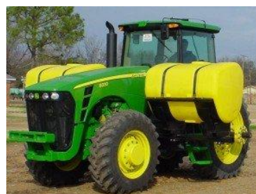
Figure 7: Tractor mounted latex tank with PTO driven latex pump.
